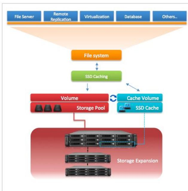
The SSD transmission speed is high, but the unit cost is higher than that of the hard disk drive (HDD). Using the SSD cache technology, we can significantly improve the IOPS and I/O speed, and maintain a relatively low unit cost in order to satisfy the demand for utilized space and transmission speed.
