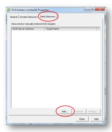
Enter the IP address of your NAS and the iSCSI target name that you created previously. In this example, enter "iqn.2004-04.com:NAS:iSCSI.ESXDataStore02.BBA3D9".
