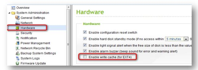
The write cache setting is disabled by default in the NAS firmware version 3.2.1 while it is enabled by default in the previous firmware versions.
